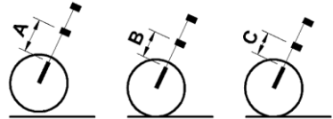
S2.1 - sag measurements front
